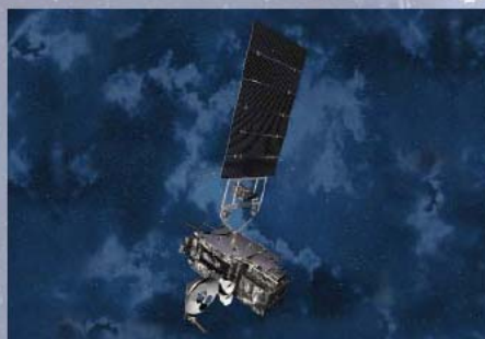
Mass < 2800kg, Size ~ 5.5 meters, Power > 4000W Image courtesy of Lockheed Martin
