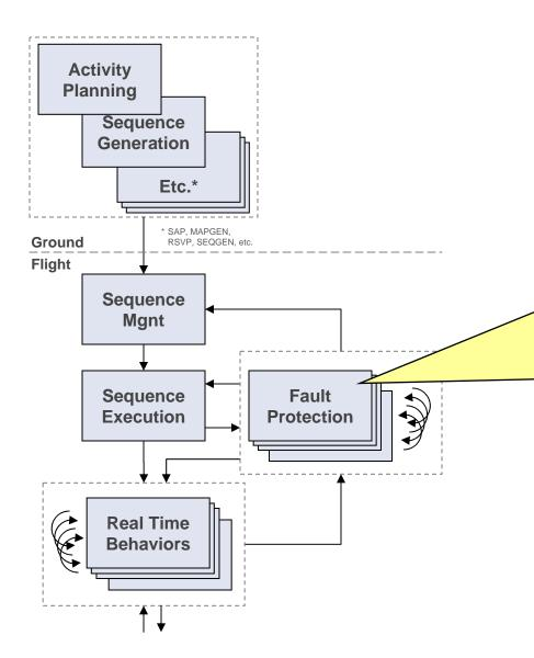
Fault protection software running in parallel, ready to "take over" from nominal sequence execution when a fault monitor is triggered. The usual off-nominal response is "safe mode":
