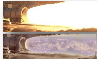
SSC HiDyRS-X (High Dynamic Range Stereo-X) is advancing with other funds and commercial partnerships. Currently working to integrate it onto a single mask/imager system.
