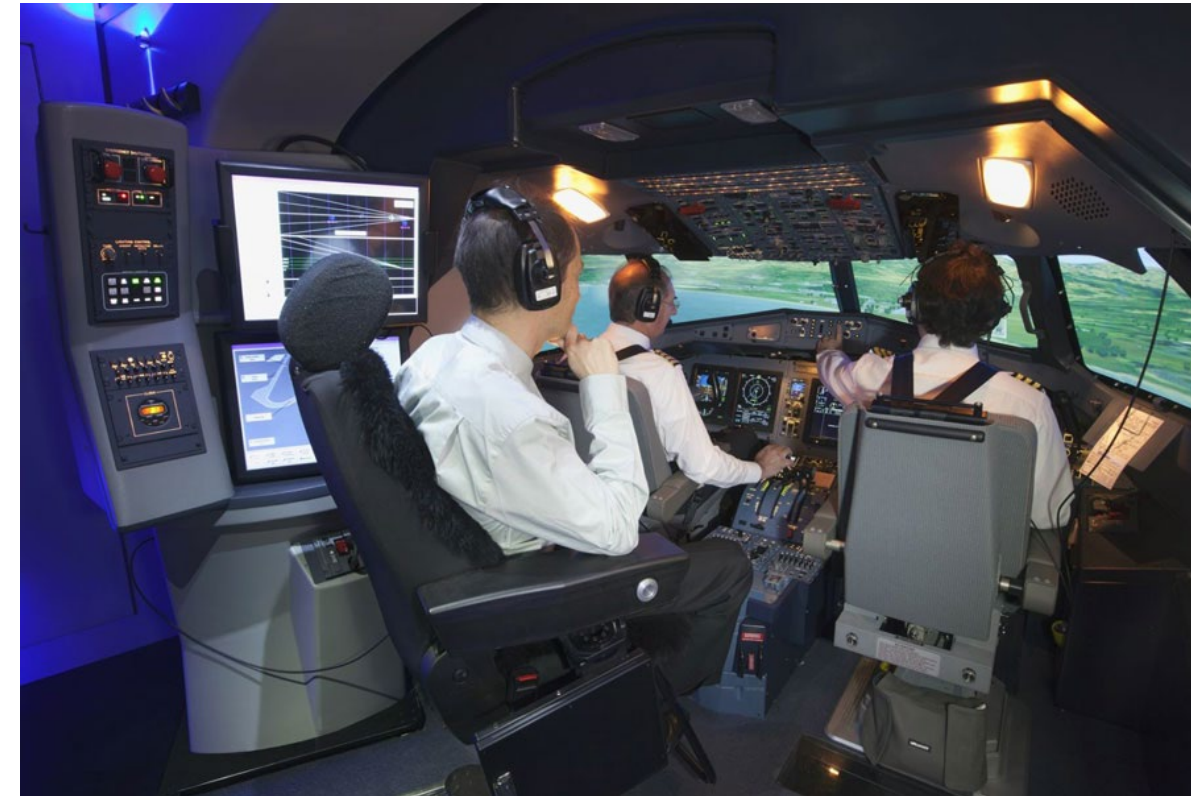
ATR 600 Flight Simulator with Instructor Station, https://www.ainonline.com/
