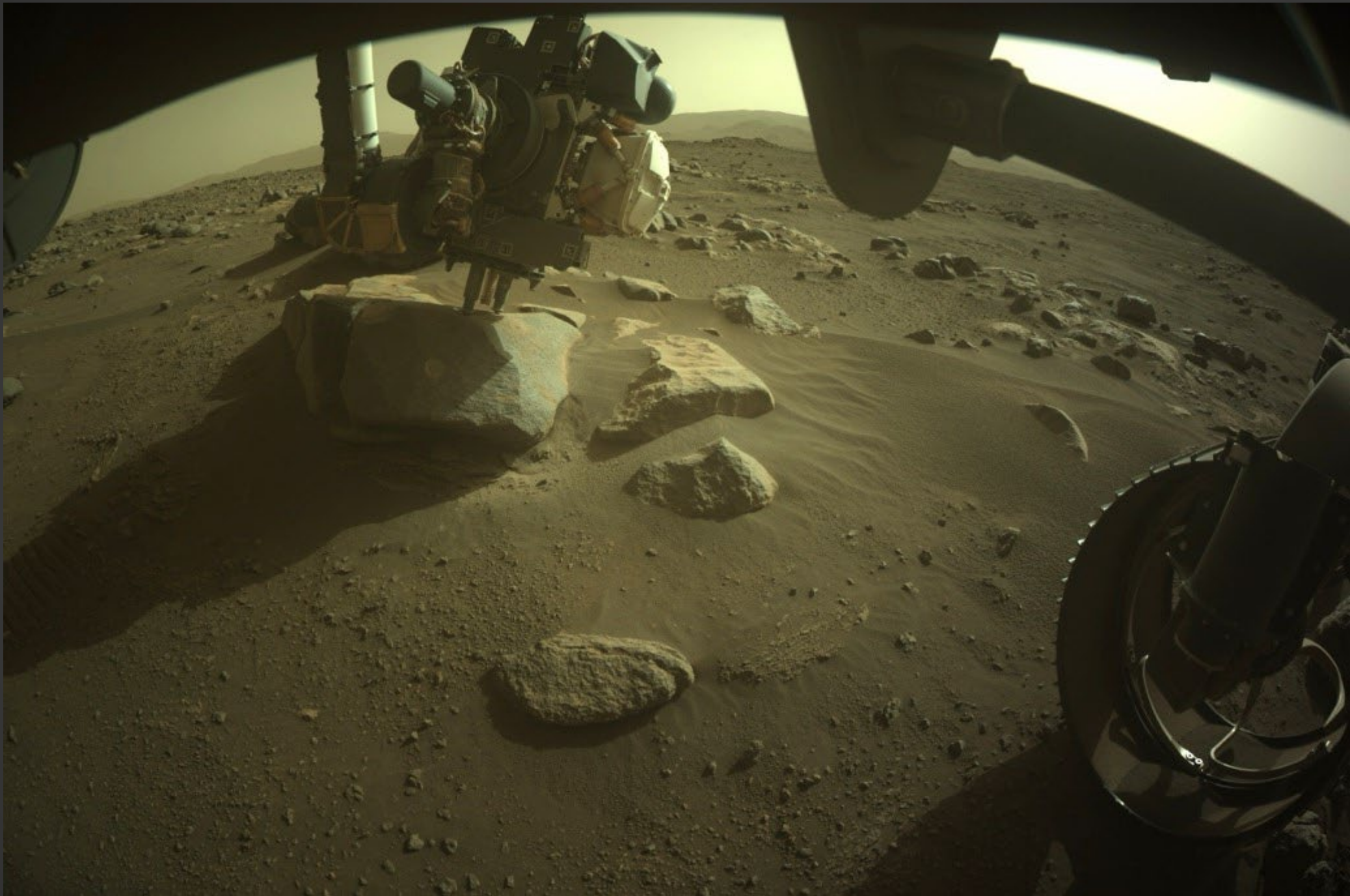
Front HazCam image of sampling the Ch-1 member ( Hahonih ) NASA/JPL- Caltech
