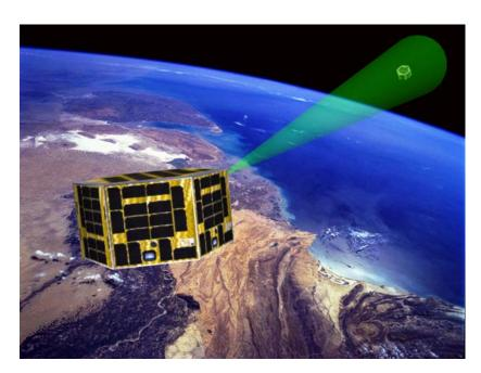
CUSat demonstrates an end-to-end autonomous on orbit inspection system. Centimeter-level accurate Carrier-phase Differential GPS (CDGPS) enables CUSat to navigate and use its cameras to gather targetsatellite imagery. In the Ground Segment, image-processing techniques verify the CDGPS relative distance and orientation estimates and provide a 3D model of the target satellite for the user.
